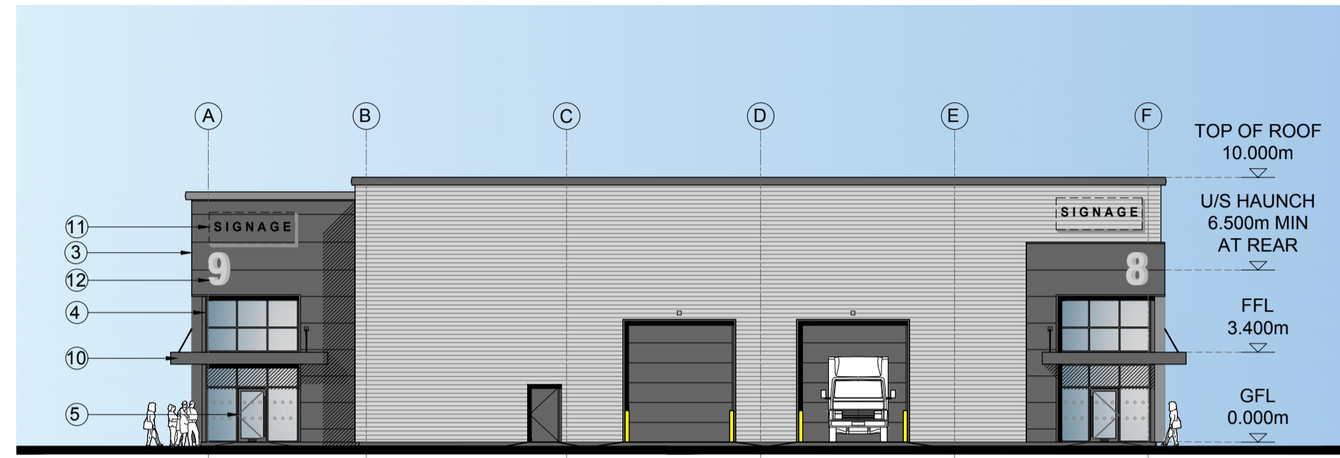
UNIT B8 - B9 NORTH WEST ELEVATION
